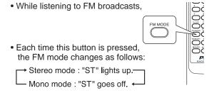
When FM stereo broadcasts are poor because of weak broadcast signals, select the FM mono mode to reduce the noise, then FM broadcasts are reproduced in monaural sound.
